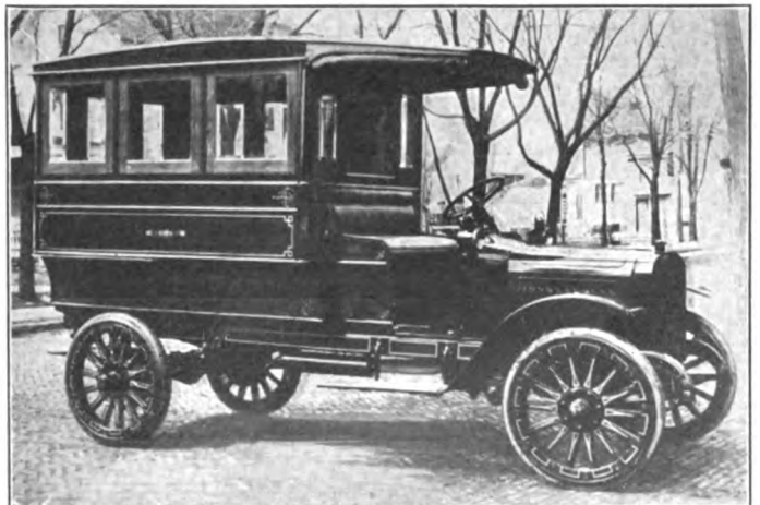
Combination Jitney and hotel bus brought out by Beck & Sons, Cedar Rapids, Iowa. It has a capacity of 2,000 lbs.
